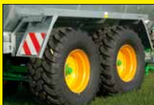
Mudguards on double axle WITH-OUT wheel recessing
