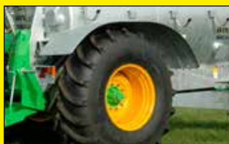
Mudguards on single axle WITH wheel recessing
