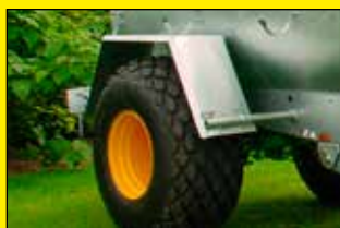
Mudguards on single axle WITH-OUT wheel recessing
