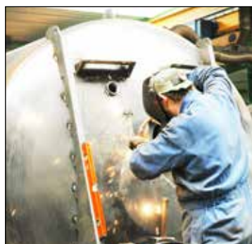
Manual welding of the accessories
